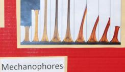
Mechanophores also have the advantage of being able to respond to stress and react to change color before failing.
