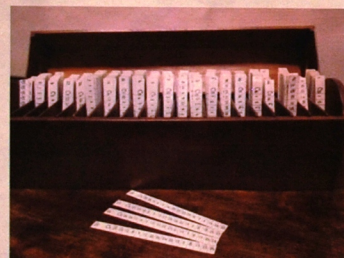
Beavers-Lipson strips, tools for calculations done by hand
