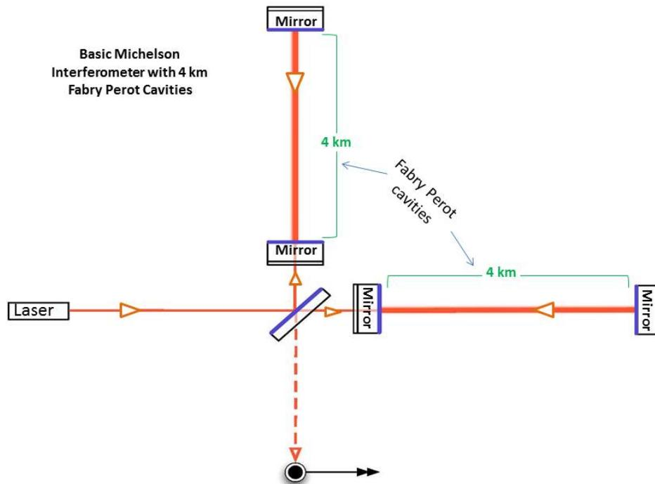
Fig. 5 “Basic Michelson Interferometer with Fabry-Perot Cavities”
