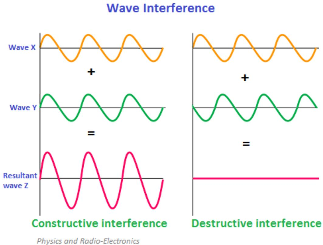
Fig. 2. “Wave Interference”
