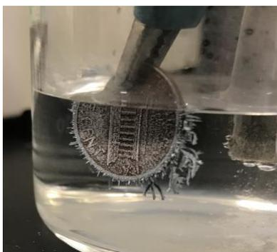
After discovering the third method was the most effective method, I used the method to collect data and observations from seven different pennies between the years 1960-2017. I electroplated each penny for 5 minutes.
