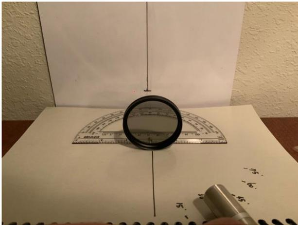
2) Experiment 2: Measure the index of refraction of various materials.
